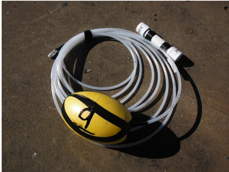
Sample station for the mooring platform prior to installation.
