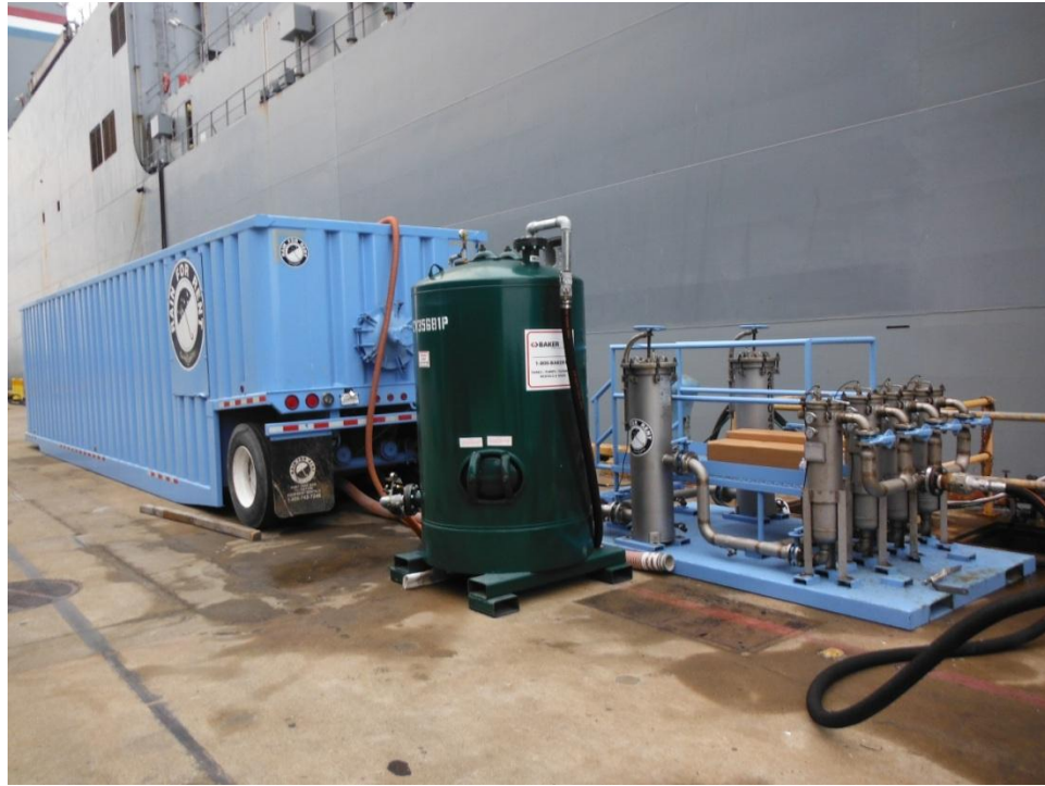
View (left to right) of the storage tank, pressure vessel, and filter cartridge array.
