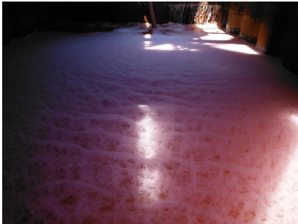
View of Tank 1 after adding rhodamine dye.
