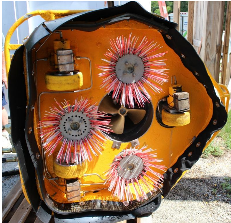
Scrubber unit with rotating brushes, suction propeller, and rubber edging.
