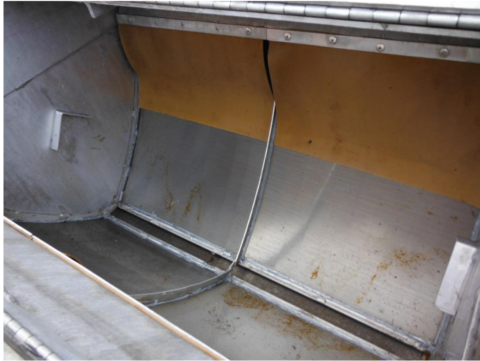
Mesh screen (100- \mu\text{m} openings) in the primary particulate filter.
